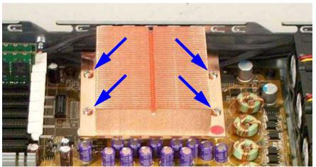
Figure 11: Removing the processor heat sink
